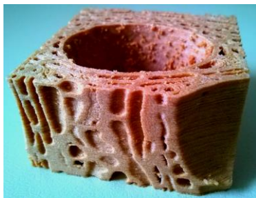
3D-printed real wood structure
