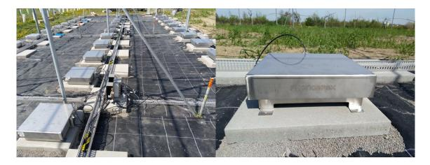
3. Plant positioning on the scales system
