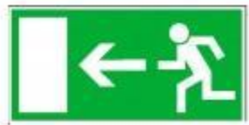
Escape Route Left
