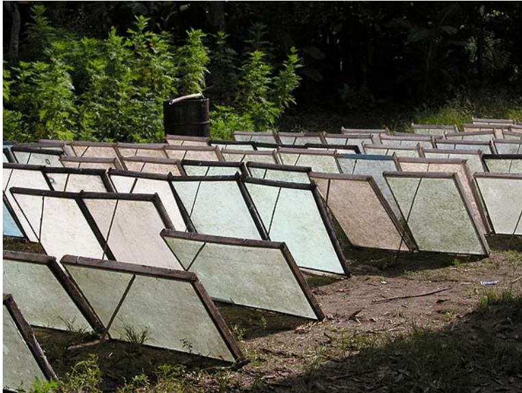
Figure 7: Mulberry paper drying on mesh screens
