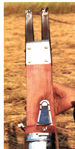
Double points of a jab-planter designed for CA.
