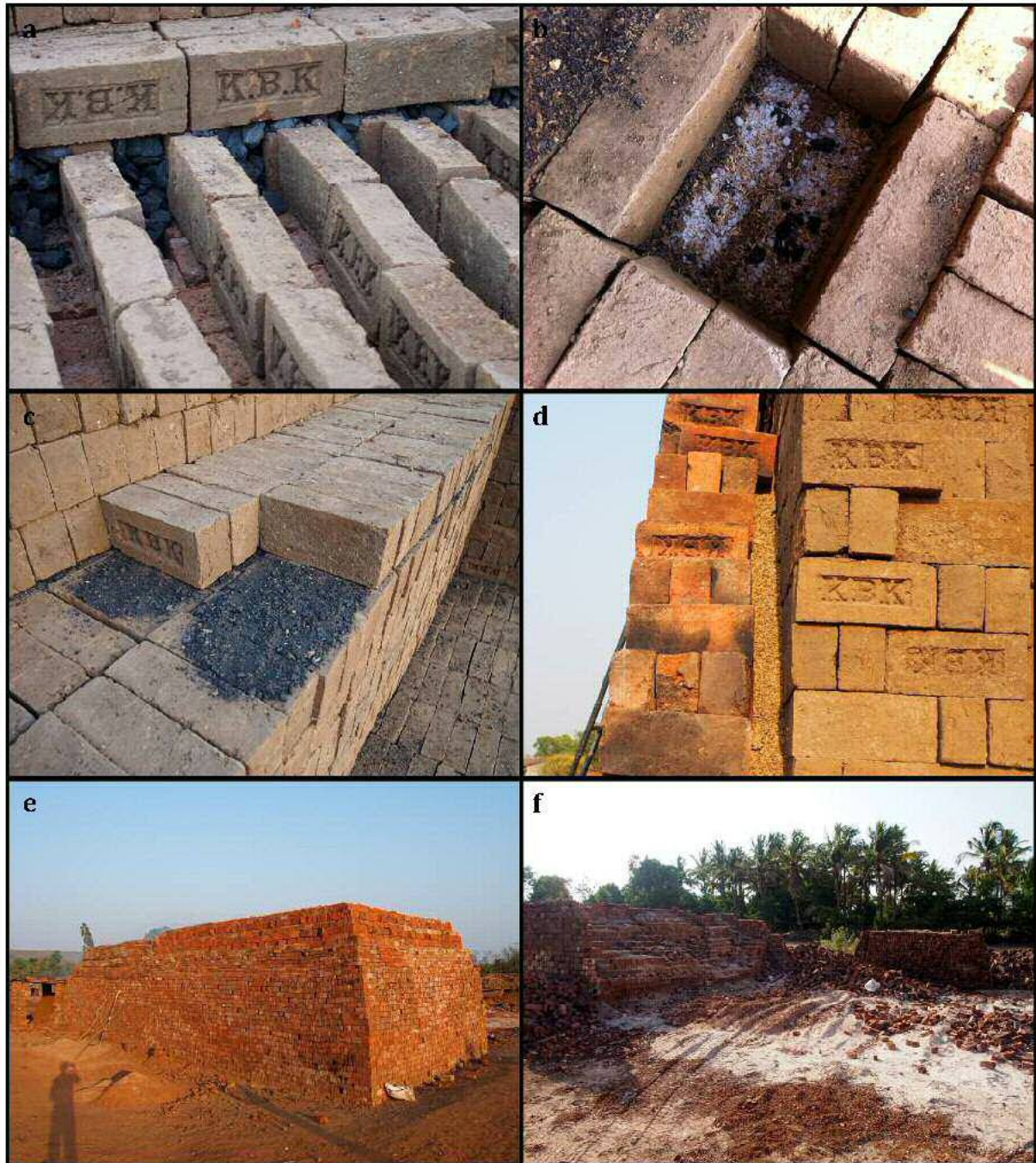
Figure 8: a) Long shafts filled with coal and enable the air circulation in the kiln b) Salt and rice husk is distributed along with coal c) Coal is distributed between each layer to guarantee the burning of all bricks d) The gap between the green bricks and the sheathing is filled with rice husk e) The piled up brick kiln ready for the burning process f) The area of the brick kiln after the burning process and removal of bricks
