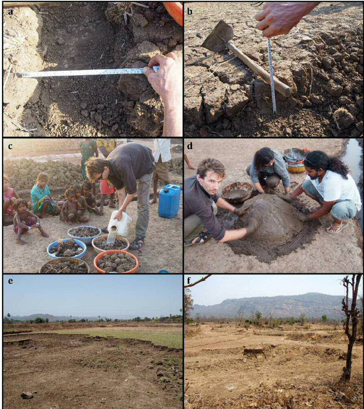
Figure 6: a+b) The extraction of 3 soil samples with a specific volume from 3 paddy fields close to the brick kiln c) Adding water to the soil samples and soak it for several hours to prepare a mouldable mass for green brick production d) Preparation of the raw mass for green bricks e) Paddy field with depleted upper layer for brick production f) Paddy fields with multiple depleted layers for brick production
