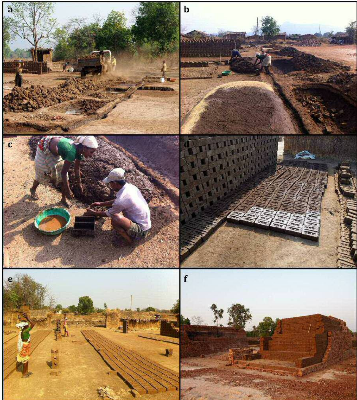
Figure 7: a) Unloading of soil from paddy fields into pits for preparation of raw material for brick production b) After 16 hours soaking with water in the pits the raw mass gets distributed next to the pits to let more water vaporize c) Moulding of bricks by hand with metal moulds d) Distribution of green bricks for the drying process in the wind and sun e) Bricks are carried to the kiln f) Brick kiln piled up with 100 thousand green bricks and a layer of burnt clay bricks as sheathing and basis
