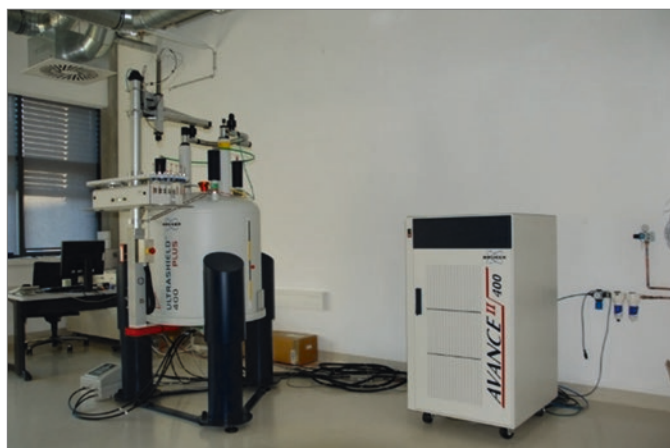
The 400 MHz instrument equipped with a liquid N 2 cooled cryoprobe (Prodigy) located at UFT
