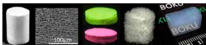
Different types of ultra-lightweight cellulosic aerogels partly covalently equipped with alloyed core/shell quantum dots.
