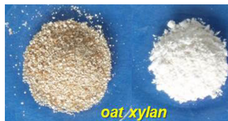
Purification of hemi-cellulose from residual lignin using scCO_2 antisolvent precipitation.
