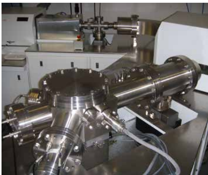
MC ICP-MS (Nu Plasma HR, Nu instruments, Wrexham, UK)
