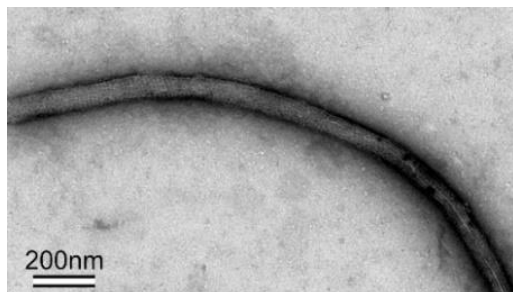
Fig.1. TEM image of an S-layer coated MWNT.
