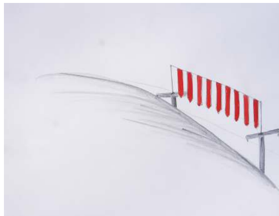
Figure 29. Plastic ties on additional cables for drag lifts.
