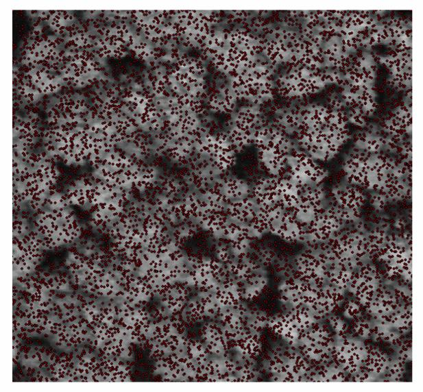
To estimate the semivariogram range, red band of spectrozonal image was sampled (mean density of 5 pts. per sq.m)
