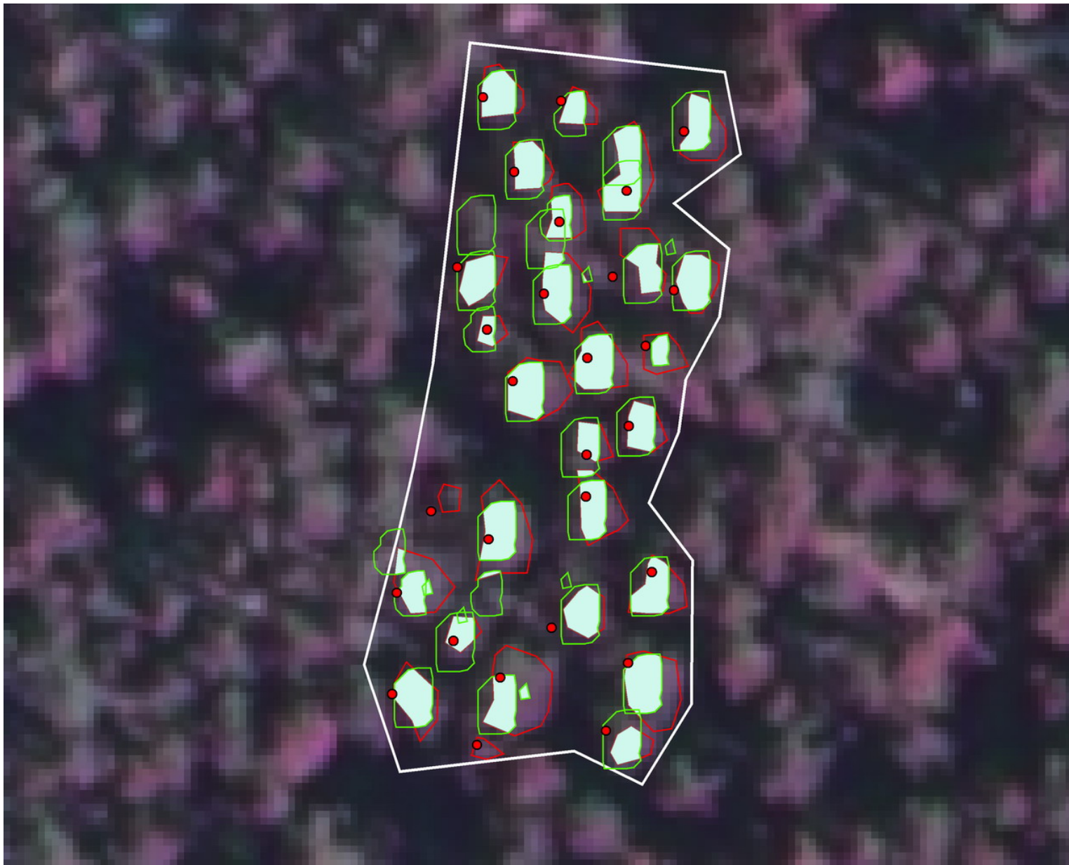
Pixel values where selected for the templates (green) that had a sufficient intersection with the manually identified crowns (red)
