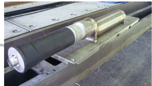
Figure 5: Modified pipe hydrophone.
