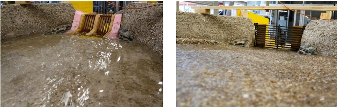
Figure 1: Screen-dam with inclined vertical beams and beam-dam with horizontal beams.
