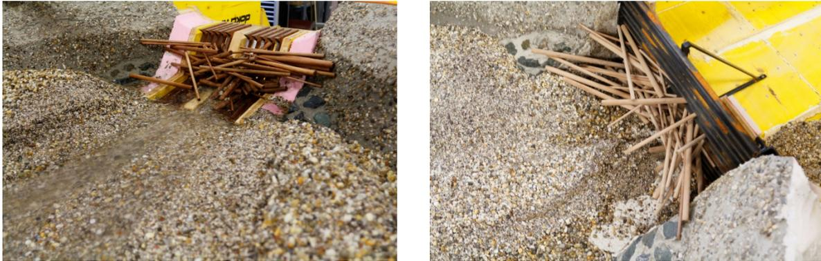
Figure 4: Example of a log jams caused by the added driftwood for both types of dams.
