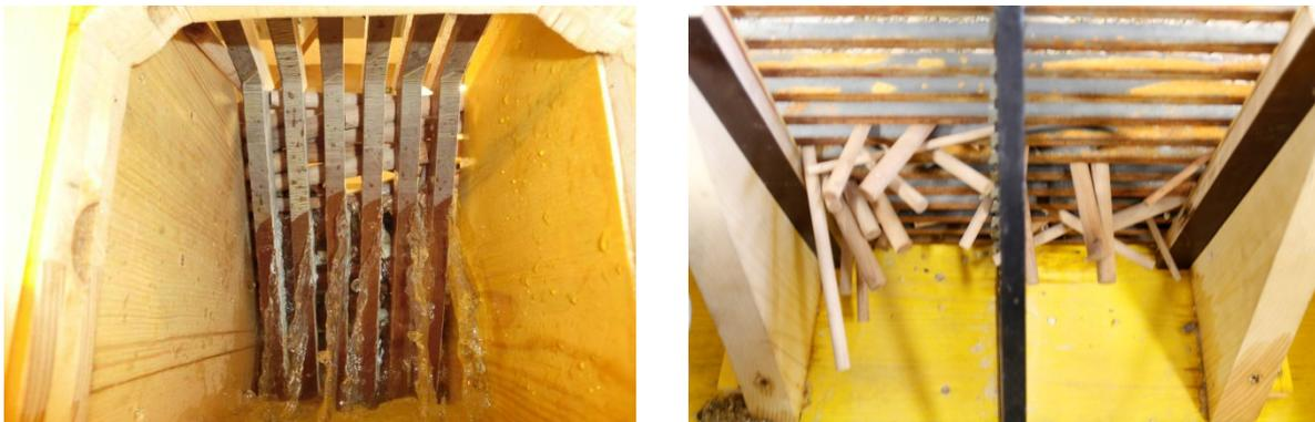
Figure 5: Rear view of log jams caused by the added driftwood for both types of dams.
