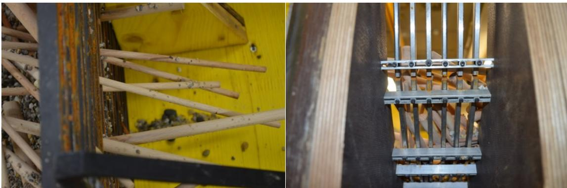
Figure 11: Different clogging behaviour of the dam types.
