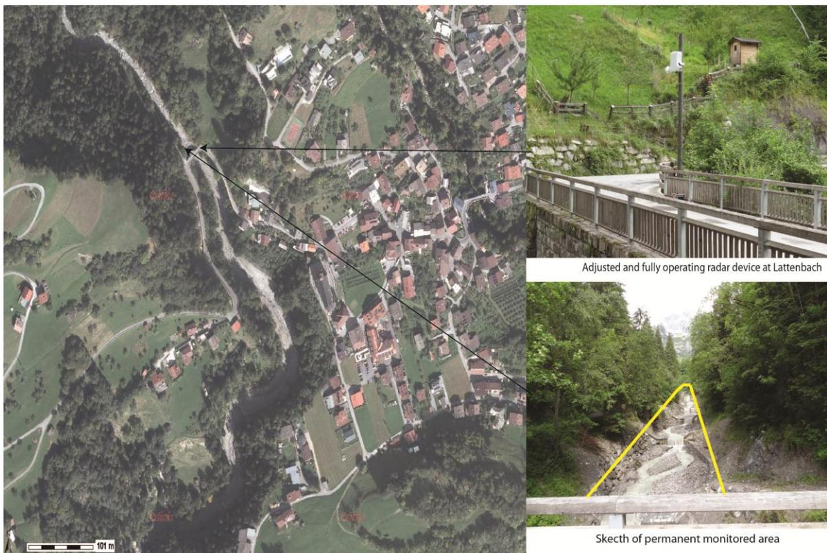
Overview of Lattenbach catchment, arrows show position of radar device and projected area (Source: tirisMaps)
