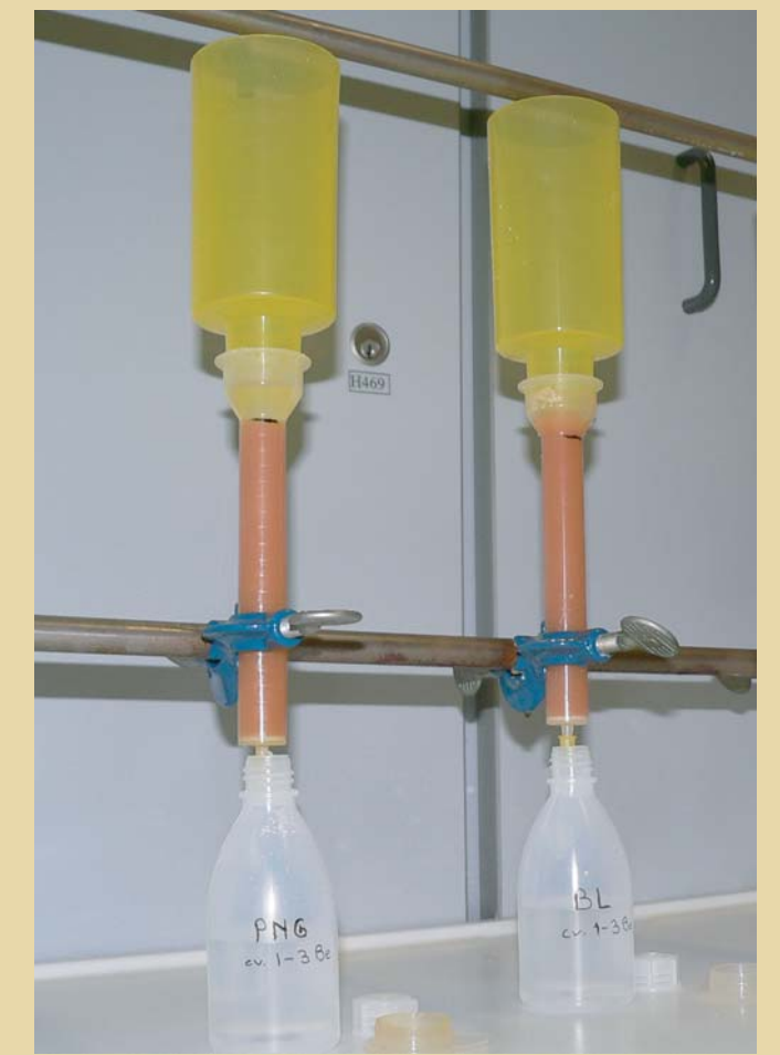
Al/Be separation by cation exchange
