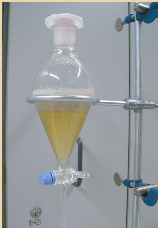
Heavy liquid separation of minerals with different density than quartz (~2.65 g/cc)
