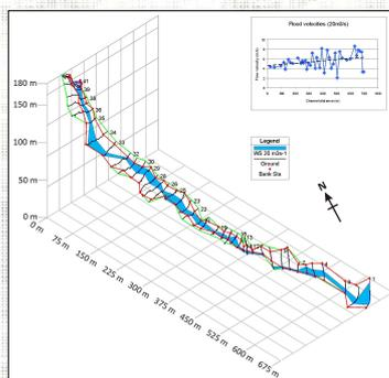
Perspective view of model output for a discharge of  $20 \text{ m}^3 \text{ s}^{-1}$  (nb. contained well within bank)
