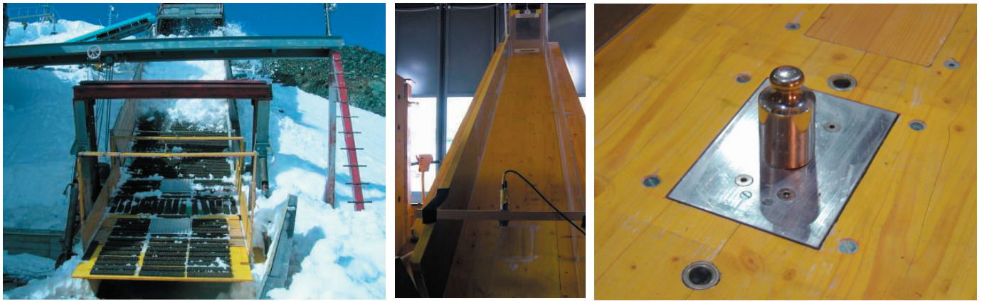
Figure 1: Large scale chute experiments with snow (left) and laboratory chute experiments with granular materials are used to measure basal shear stresses S and normal stresses N (middle). The chutes are instrumented with shear and normal force plates and optical flow height sensors (right).
