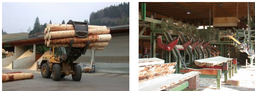
Fig 7 - "Heavy wood & heavy equipment" - transport, conveying and logistics of large dimensioned wood in a saw mill are special challenges (source: R. Stingl, ihf/BOKU)
