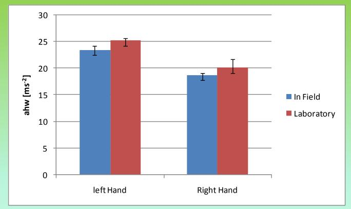
Comparison of a<sub>hw</sub> values for both hands in laboratory and in-field tests
