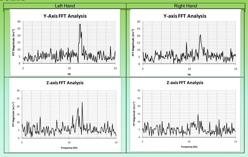
FFT spectrum for the Y and Z axes for both hands.
