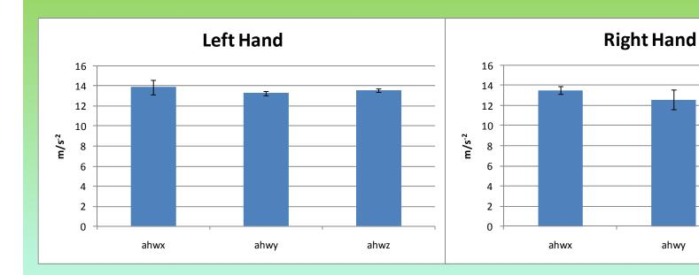
The resulting weighted vibration level for each axis
