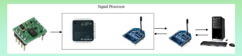
The experimentation allowed to gather and characterize the vibration data, in terms of frequency spectrum and intensity. Such information has been subsequently exploited for real-time vibration monitoring and subsequent health hazard assessment. The transmission was performed via wireless network to a station where the data were stored and analyzed.
