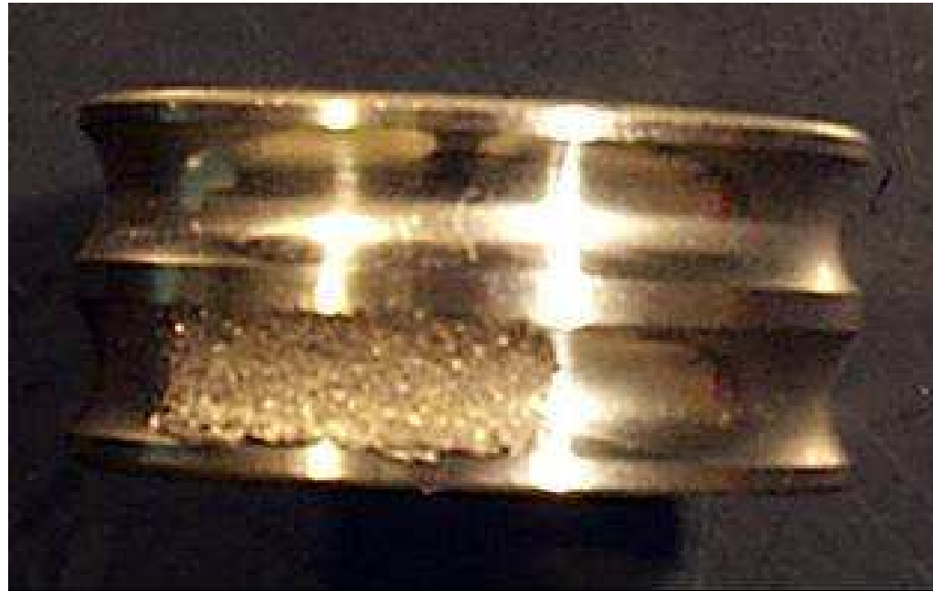
Example of an extended fault in the inner race.
