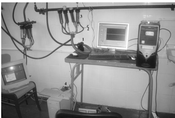
Figure 8: General view of the testing systems 1-electromagnetic pulsator; 2-pressure transducer; 3-tested teatcup; 4-computer driven pulses generator.
