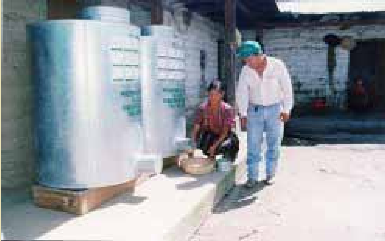
Galvanized steel silo
