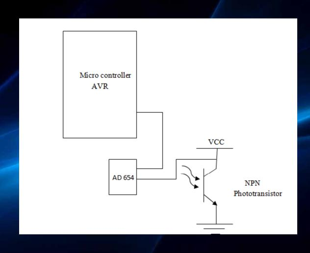
A light intensity controller circuit was designed and incorporated in the platform. This circuit included a photo-transistor, a V-F convertor (AD654 IC) and a microcontroller. As the phototransistor senses the light, it emits voltage which is converted to frequence by a v-f circuit. The Microcontroller periodically counts the output frequency. If the frequency was lower than a specific level (in this study 30000 HZ) an alarm LED will switch on as a sign for immediate remedy.`
