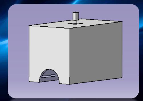
• For illumination purposes six white LEDS were accommodated on the top inner side of the platform. The LEDs were used to avoid flicker effects. To prevent shadow and also to strengthen the light, the inner walls of the platform were white painted.
