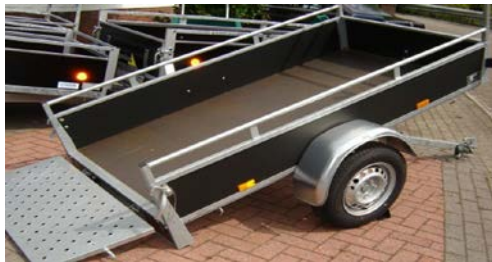
Trailer loading-panel made from hemp-flax
