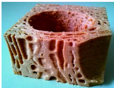
3D-printed real wood structure
