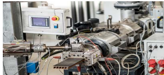
Profile-extrusion with co-extrusion using natural materials / residues
