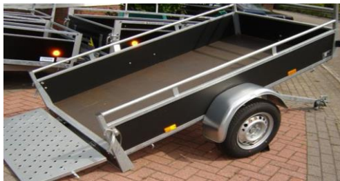
Trailer loading-panel made from hemp-flax
