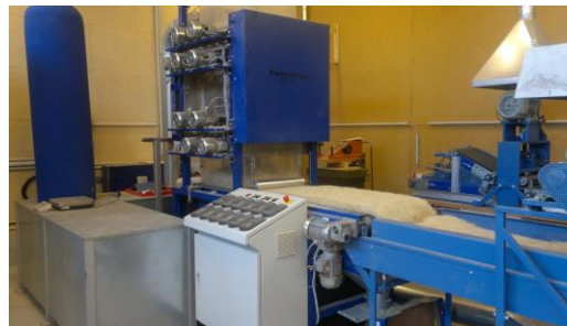
SPIKE –air-laid natural fibre fleeces
