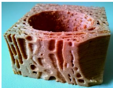
3D-printed real wood structure
