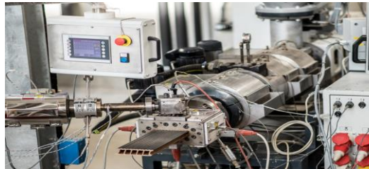
Profile-extrusion with co-extrusion using natural materials / residues
