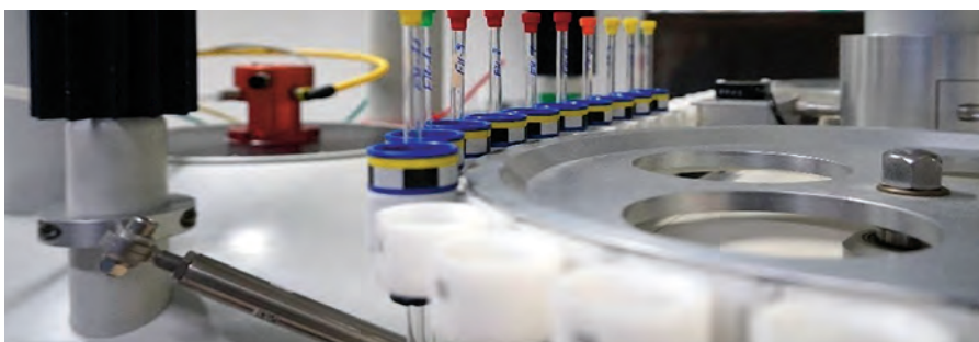
Advanced lignin analysis: lignin samples in the autosampler waiting to be analyzed by nuclear magnetic resonance spectroscopy (NMR).
