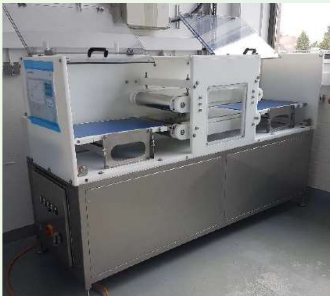
Continuous prototype for thawing of frozen food in blocks (30 kW)
