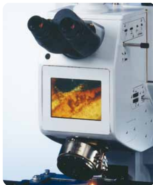
Integrated LCD screen on the HYPERION makes the sample positioning and the identification of the region of interest more comfortable.
