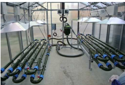
Figure Tubular photobioreactor at pilot scale for photoautotrophic PHB-production by Synechocystis cf. salina .
