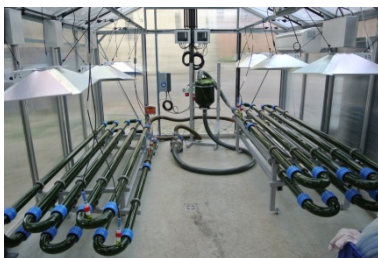
Figure 1 Tubular photobioreactor at pilot scale for photoautotrophic PHB-production by Synechocystis salina
