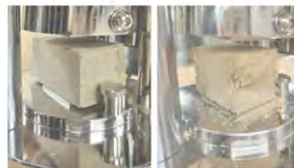
Fig. 4 compressive strength test set up according to standard EN 1015-11
