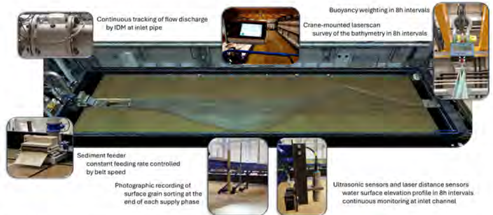
Figure 3. Measuring equipment and data collection methods
