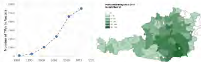
Figure 3: Development of implemented VF wetlands \leq 50 PE in Austria (left: data from Langergraber, 2018) and number of VF wetlands per district in 2016 (right: Langergraber, 2018).
