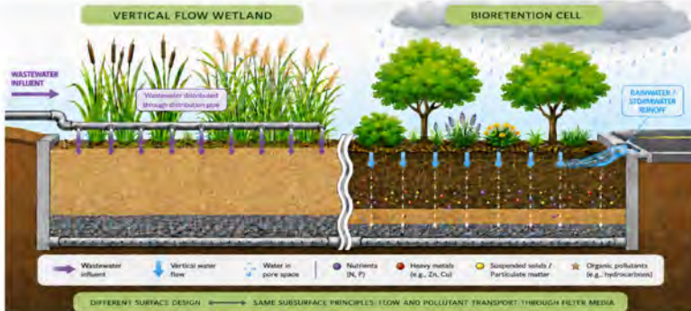
Fig 1. Illustration of a Bioretention Cell and a vertical flow wetland, showing the similarity of the systems
