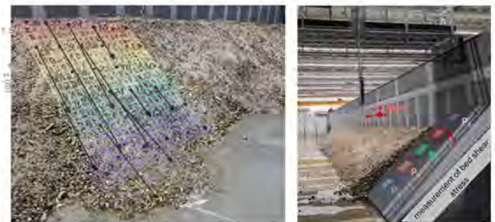
Figure 2: Left: tracer stones and their analyzed movement patterns. Right: measurement system integrated into inlet structure, consisting of five independent force plates for measuring shear stresses along the bank slope.
